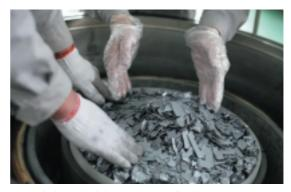
Scrap polysilicon is loaded into a monocrystalline furnace.
